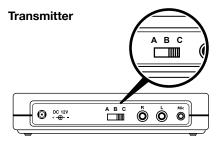
NOTE: If the transmitter is switched to another channel, the receiver also has to be set to the same channel.
