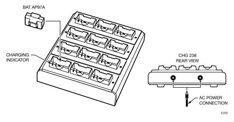
1. Plug the TFP 024 power supply into the AC wall outlet. Plug the power connector into either jack on the rear of the CHG 238 unit (above).
