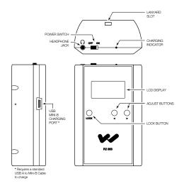
Power on the receiver(s) by sliding the power switch from "OFF" to "ON" position (Fig. D). The display will light up and show the current channel, headphone
